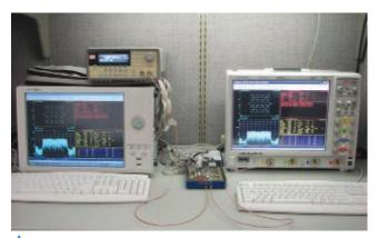
▲ Fig. 2 Mixed-signal SDR test setup using a logic analyzer with dynamic probe and VSA software and a digital oscilloscope with VSA software.
