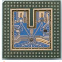
▲ Fig. 3 Agilent's DSO-X front-end module with preamp based on the HB2B InP HBT process also contains the trigger and sampler ICs.
