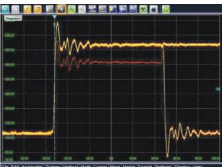
▲ Fig. 5 R&S rapid acquisition capability provides a "persistence" view of rare signal behaviors in this example of a random runt pulse.
