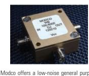
Modco offers a low-noise general purpose amplifier. Model Number WB100-6000DJ covers a frequency range of 100MHz through 6000MHz. The amplifier is housed in an Iridite Gold finished aluminum housing measuring 1.25" x 1.25" x 0.60". It is supplied with three SMA F Connectors. The device operates from a single +5V supply and consumes 60mA
