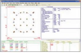
Fig. 7 LTE OFDMA MIMO VSA demodulation results.
